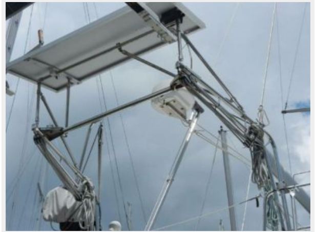
Davits and solar panels
