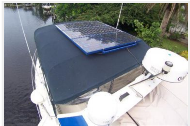
450 Watt Solar Panel Array
