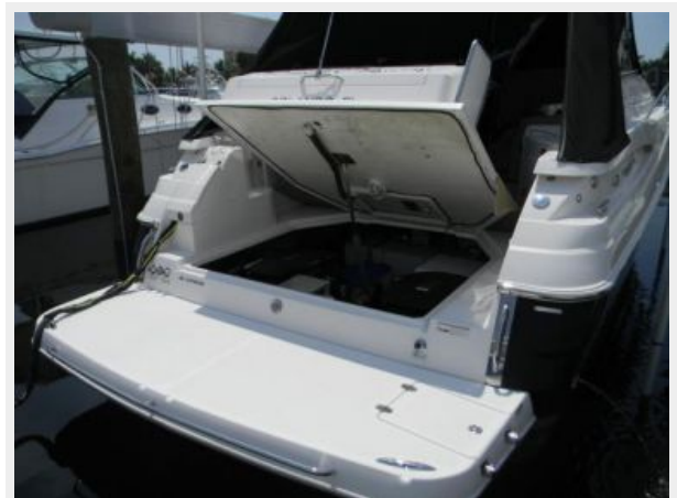
Engine Room Access
