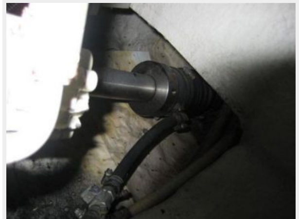
Starboard Dripless Stuffing Box
