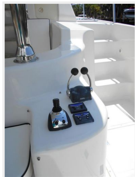
Aft Deck Control Station
