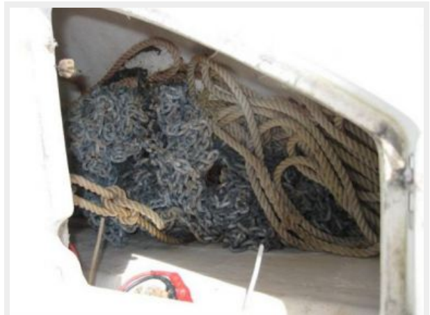
Anchor Rode Locker
