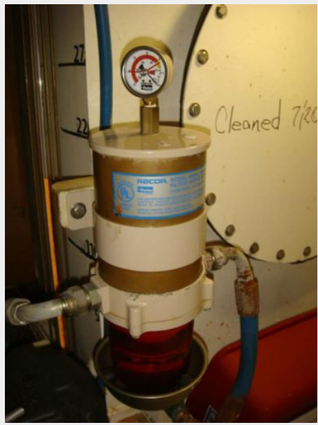
39' Neville Trawler Racor fuel filter
