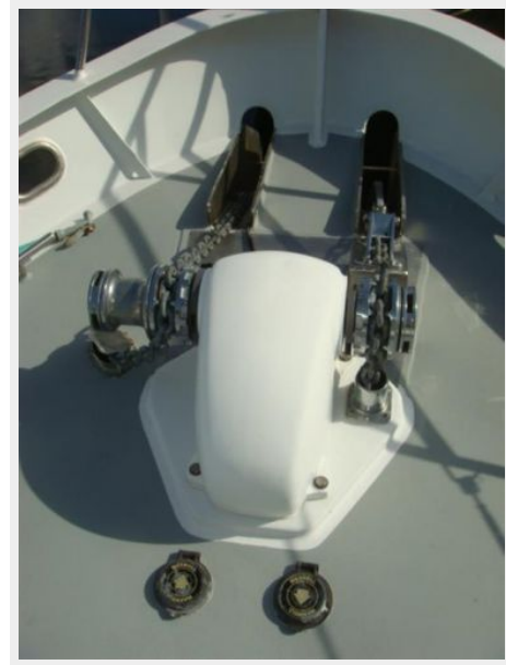
39' Neville Trawler anchor windlass
