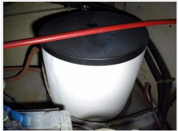
36' Chris Craft Water Heater
