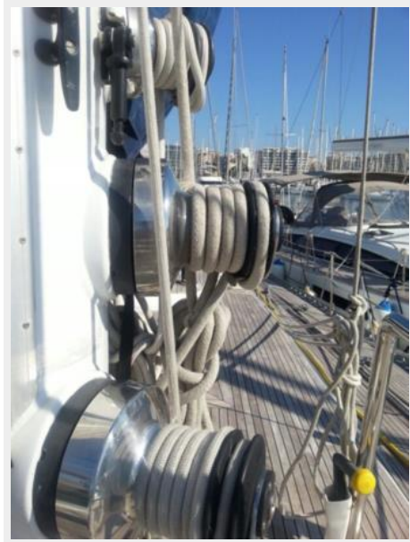
Winches on mast
