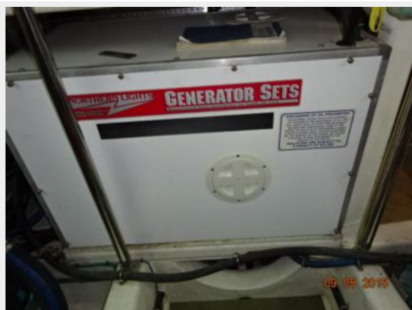
54' Ocean Alexander generator1 sound box
