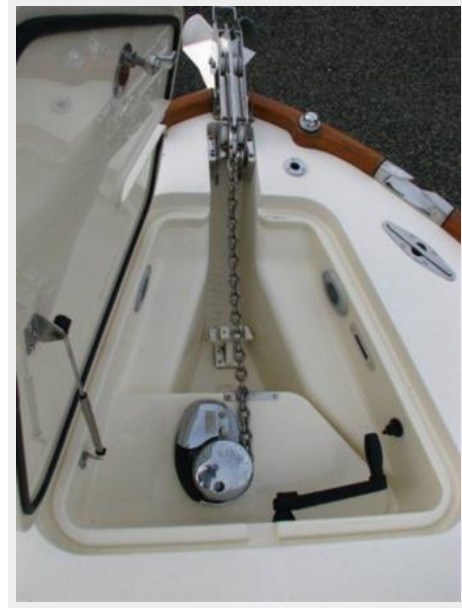
Deck 1 - Anchor Locker
