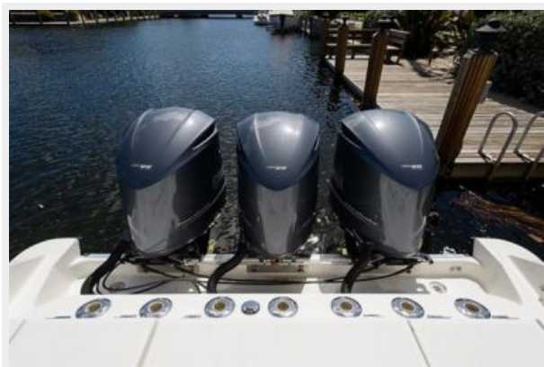
Triple Yamaha F350 4 Stroke V8
