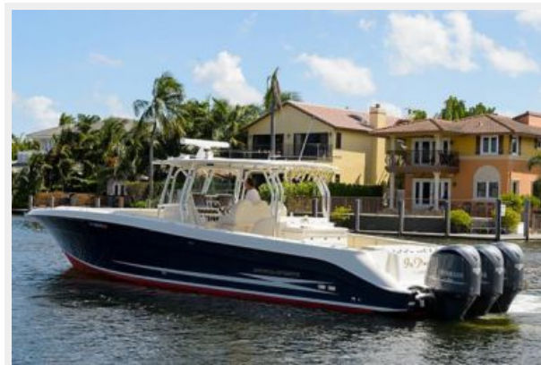
Triple Yamaha F350 4 Stroke V8
