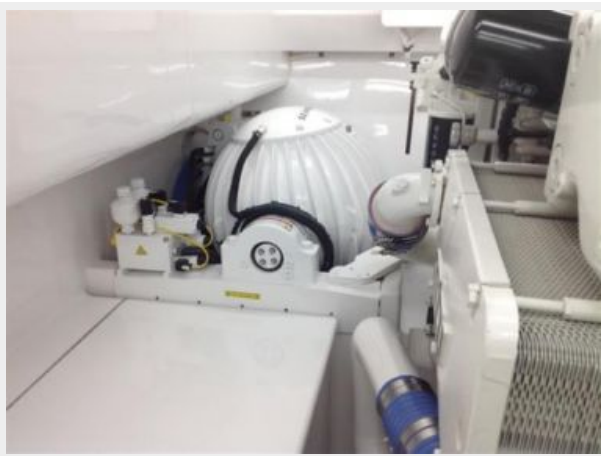
Engine Room - Seakeeper Gyro Starboard
