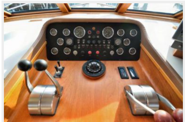
Lower Helm Controls
