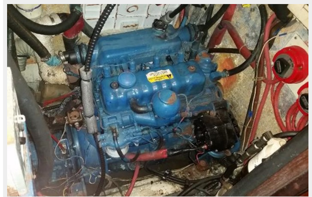
Perkins 4-108 Diesel - 50HP (1300 hrs.)
