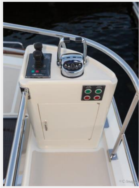
Bridge Deck Docking Station
