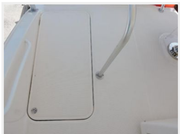
Access hatch for ladder or stairway to flybridge
