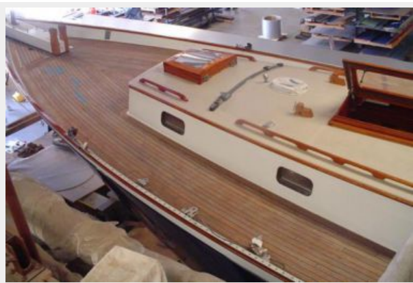
Forward Top Deck - NEW TEAK DECKS
