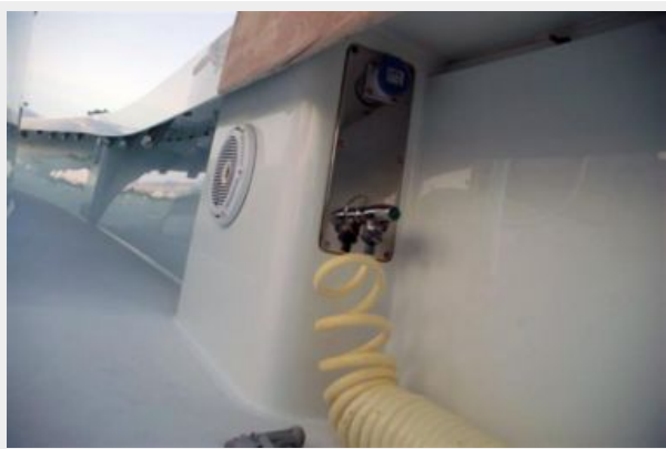
washdown hoses, speakers around side decks
