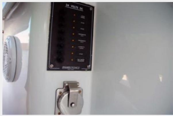
panels for exterior/underwater lights, mascerators, washdown pumps
