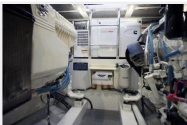
Cummins/Onan generator, oil change system
