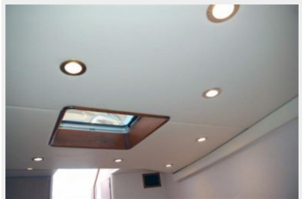
overhead hatches, LED lighting
