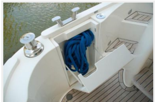
Line storage compartments and warping winch
