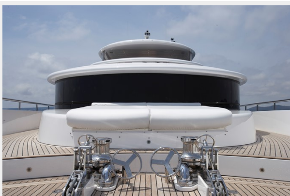
Twin anchor system
