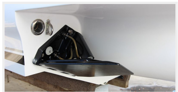
Mercury K-Plane Trim Tabs W/Mechanical Indicators
