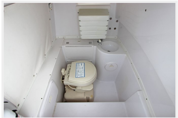
Center Console Head W/Sink, & Dometic Marine Head W/Macerator & Pump-Out
