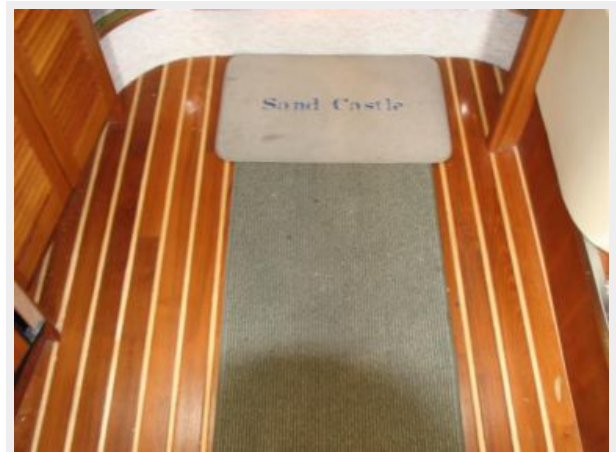
Main Cabin 4 - Teak & Holly Floor
