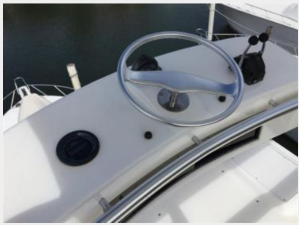
Tower Control Box w/Steering and Eng Controls
