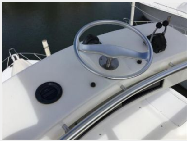
Tower Control Box w/Steering and Eng Controls
