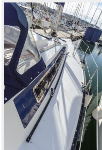
Starboard deck (new window s/s treatment)
