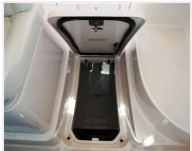
Day Hatch to Engine Room
