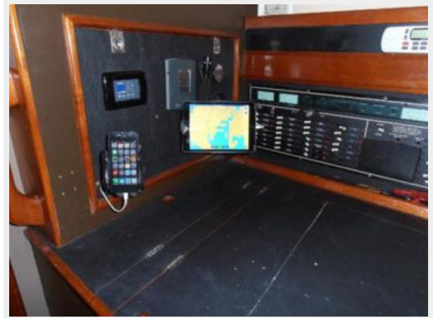
Navigation Station & AC/DC Panel
