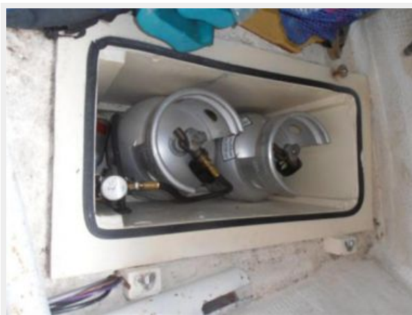
Two 10lb S/S Propane Tanks In Sealed Locker
