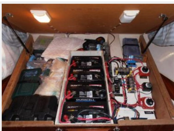
Main Bank of Batteries Under Queen Berth
