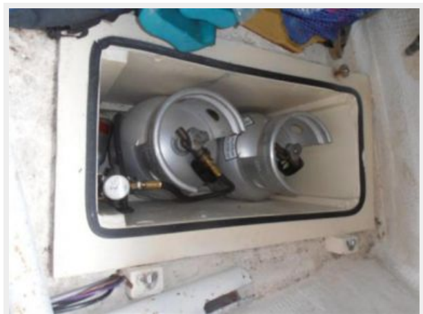
Two 10lb S/S Propane Tanks In Sealed Locker
