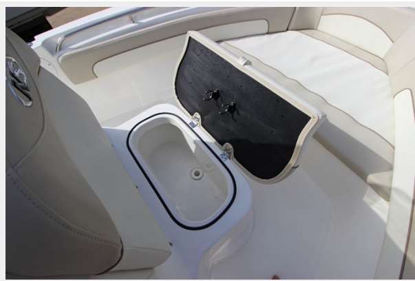
15-Gallon Insulated Cooler Under Forward Center Console Seat
