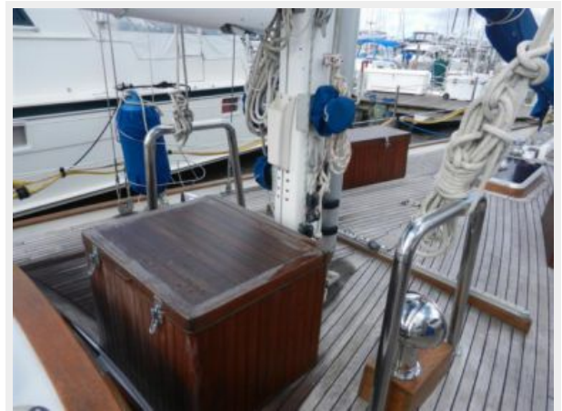
SS Safety bars at main mast
