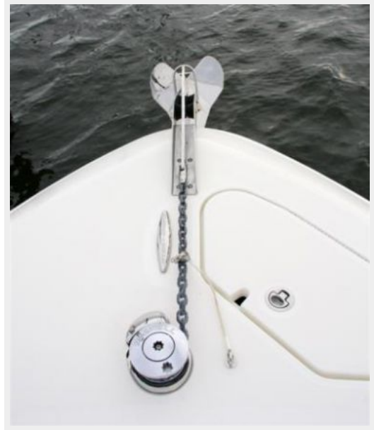
Anchor & Windless with Safety Cable
