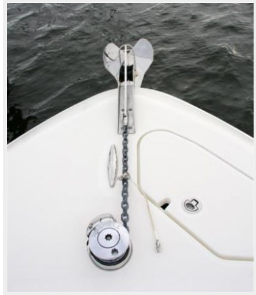
Anchor & Windless with Safety Cable
