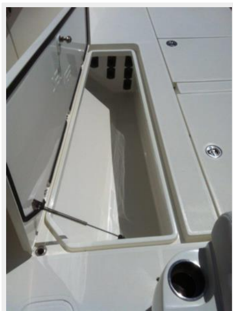
Rod storage underdeck side hatch
