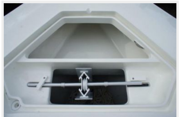
Anchor and fender storage
