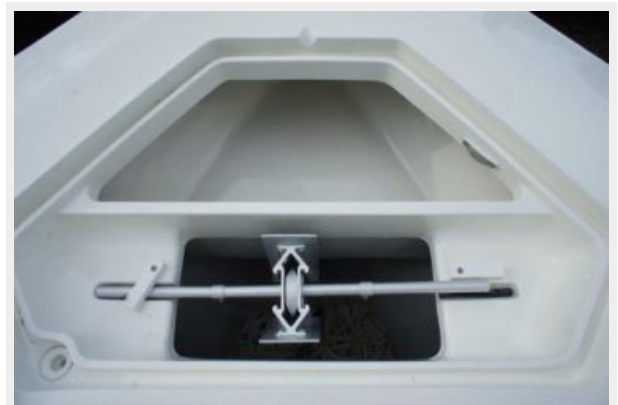
Anchor and fender storage
