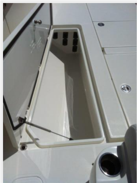
Rod storage underdeck side hatch
