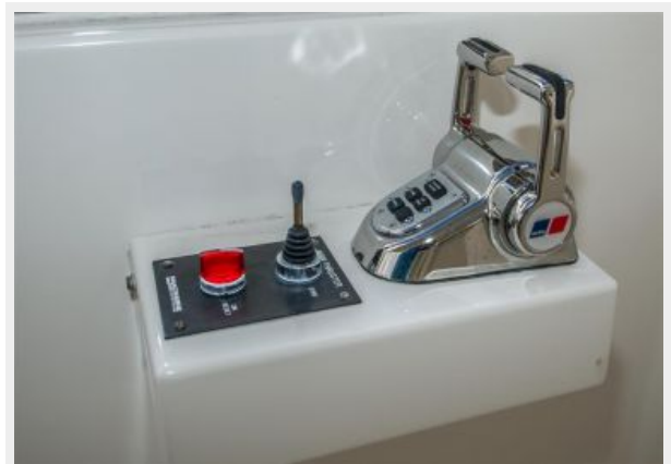
Flybridge Wing Controls
