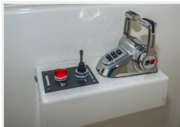
Flybridge Wing Controls
