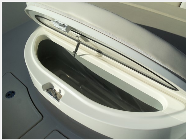
Insulated Cooler Well
