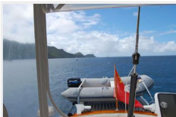
RIB Dinghy on TNT lift
