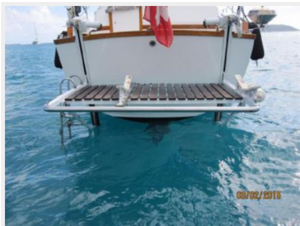
Swim Platform on TNT lift
