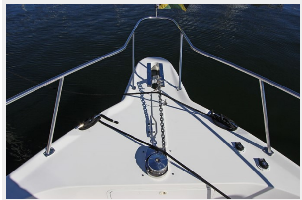
Bow Pulpit W/Electric Windless Anchor & Stainless Railing
