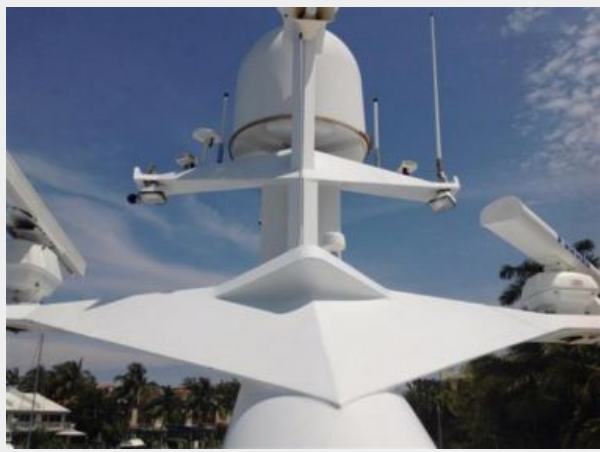
MAST - Sat Com Dome
