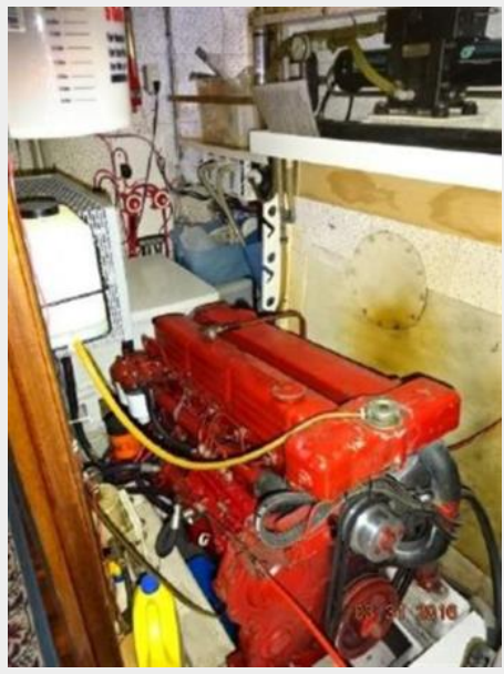
50' Marine Trader port engine room aft
