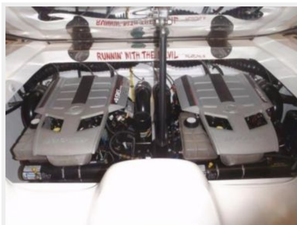
Engine Room Mercury 496 HO
