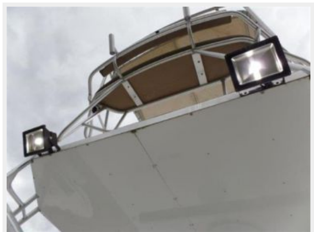
Cockpit Flood Lights
