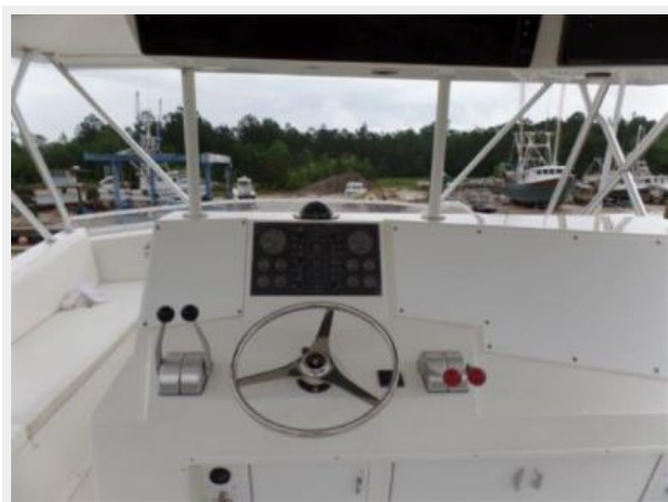
Helm Control Station
