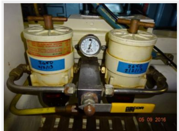
49' DeFever port Racor fuel filters
