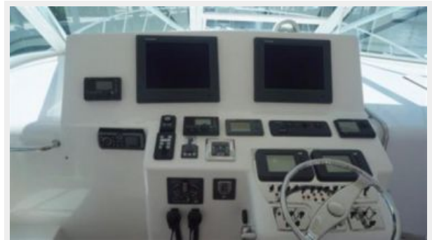
Bridge Console with Cat Controls, Furuno Chartplotter Screens, Auto Helm, Bow Thruster, Sirius Radio, VHF's, Yacht Controller
