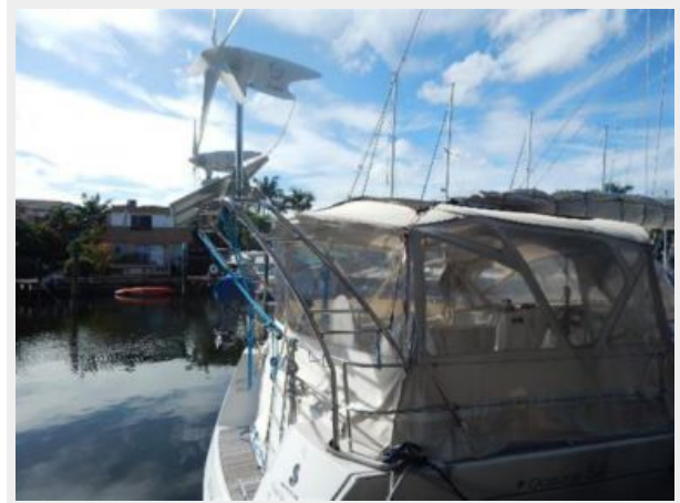
Stern Arch - (2) wind generators
