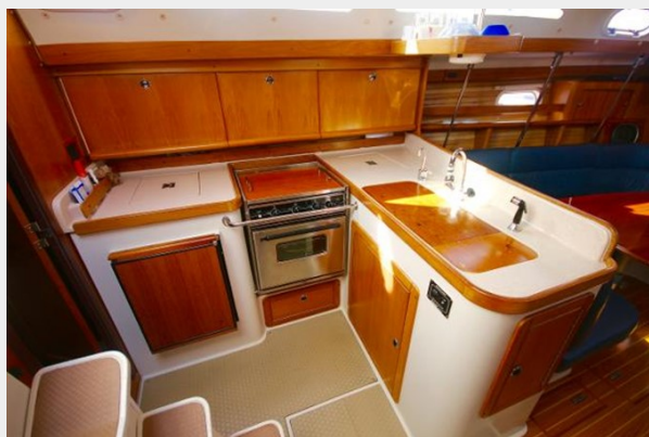
Galley - The L shaped galley was designed to be safe even while underway.
