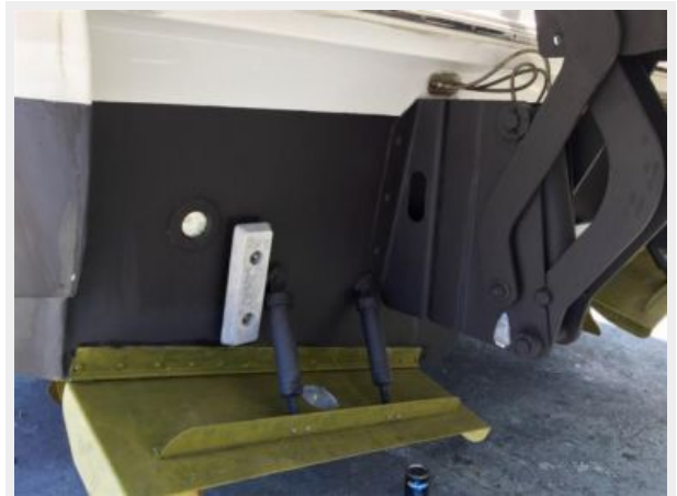
Fresh Bottom Paint and Zincs - 2016
